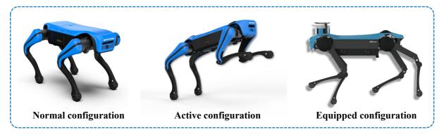
Figure 4-2 Three type of action configuration of the proposed robot
