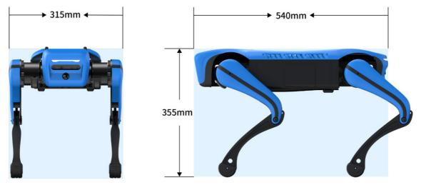
Figure 4-1 Configuration dimensions of the quadruped robot
